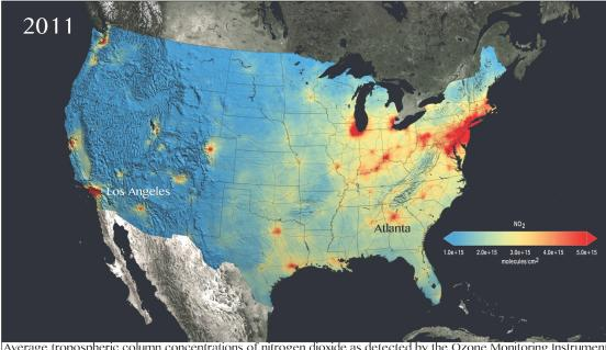
Average tropospheric column concentrations of nitrogen dioxide as detected by the Ozone Monitoring Instrument on NASA's Aura satellite for 2011. Blue and green denote lower concentrations and orange and red areas denote higher concentrations, ranging from 1e+15 to 5e+15 molecules per square centimeter, respectively. Image credit: NASA Science Visualization Studio. 1. Have tropospheric  $NO_2$  concentrations increased or decreased from 2005 to 2011 in the following cities?
